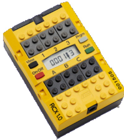
Figure 2: The LEGO RCX can power up to 3 outputs and accept inputs from 3 sensors
